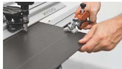
2. Cutting of Tile
